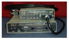
Figure D- 2. Data logger controller & cable adapter box
