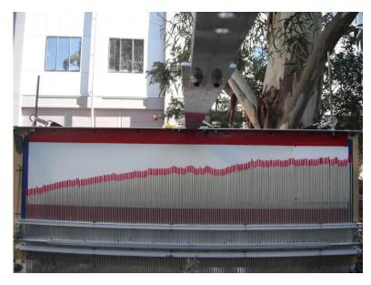
Figure 7-5. Pin profiler for surface roughness measurements.
