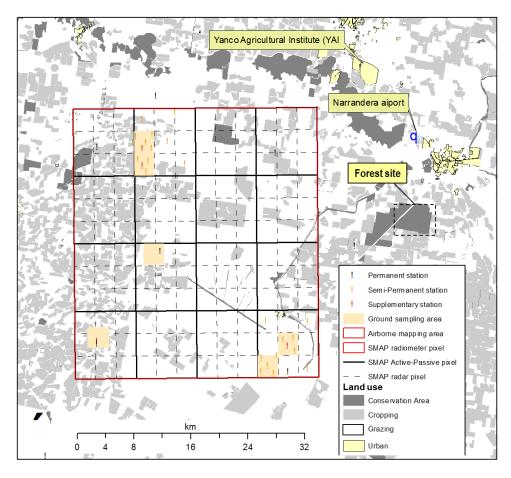
Figure 1-2. Overview of the SMAPEx-3 experiment. The map shows the area covered by airborne mapping (red rectangle), the ground soil moisture networks (coloured dots), ground sampling focus areas and prescribed SMAP grids for radiometer, radar, and active-passive products.
