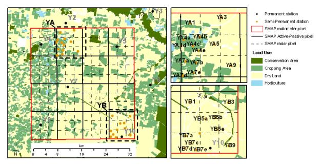
Figure 4-8. Layout of the SMAPEx semi-permanent soil moisture network in the study area.
