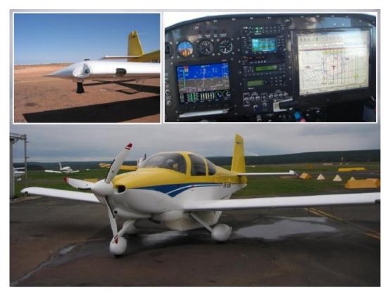
Figure 3-1. Experimental ESV aircraft showing a wingtip installation in the left inset, and the cockpit with cockpit computer display in the right inset.
