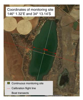
Figure 5-4. Calibration flight (red line) and boat transects (white lines) over Lake Wyangan
