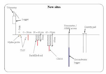
Figure 4-5. Typical equipment at the original (2001) and new (2004) soil moisture sites in the Murrumbidgee catchment. Each site provides continuous data of rainfall, soil moisture at 0-5cm (or 0-7cm), 0-30cm, 30-60cm and 60-90cm and soil temperature and accommodates periodic measurements of gravity, groundwater and TDR soil moisture measurements.
