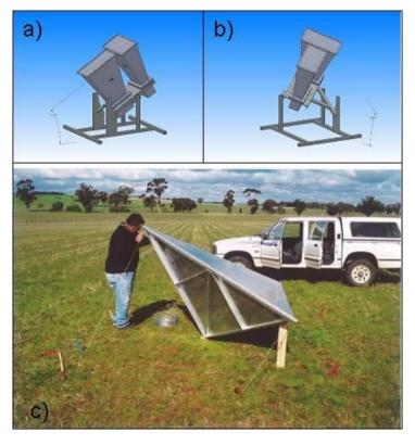
Figure 5-6. Polarimetric Active Radar Calibrators #1 and #2 (a), #3 (b) and Passive Radar Calibrator (c).
