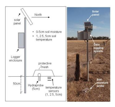
Figure 4-7. Schematic layout of the additional SMAPEx monitoring site and photo of site YA5.
