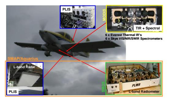
Figure 3-2. View of PLIS antennas, PLIS RF unit, PLMR and the multispectral unit.
