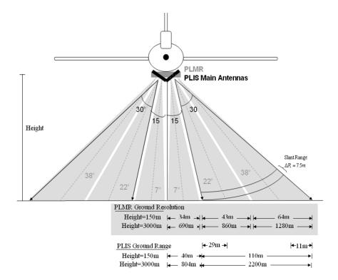
Figure 5-1. PLMR and PLIS viewing configuration on the RV-10 aircraft.
