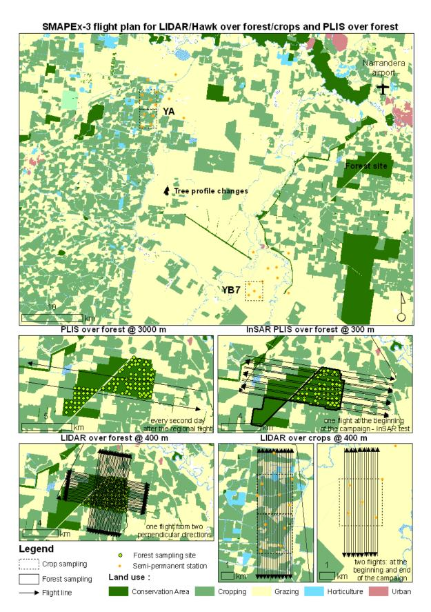
Figure 5-3. Overview of the SMAPEx-3 target SAR, InSAR, and LIDAR flights.
