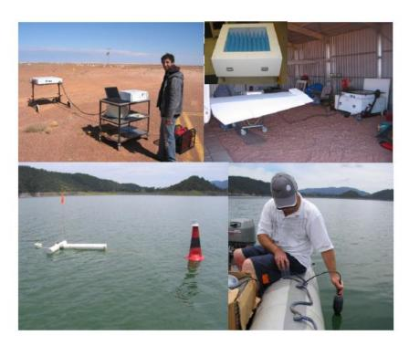
Figure 5-5. Upper left: undertaking a sky cold point calibration with PLMR; upper right: undertaking a warm point calibration with the calibration box shown in the inset; lower left: the buoy used to monitor water temperature and salinity; lower right: undertaking a boat transect of water salinity and temperature.
