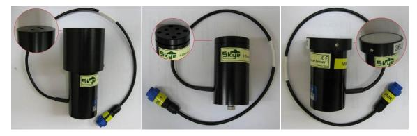
Figure 3-7. Multi-spectral sensors; downward looking sensors (left and midddle) and upward looking sensor with cosine diffuser fitted (right).
