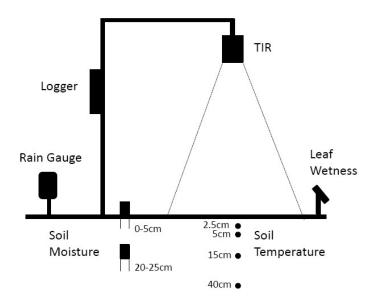
Figure 6-1. Schematic of the temporary monitoring station.
